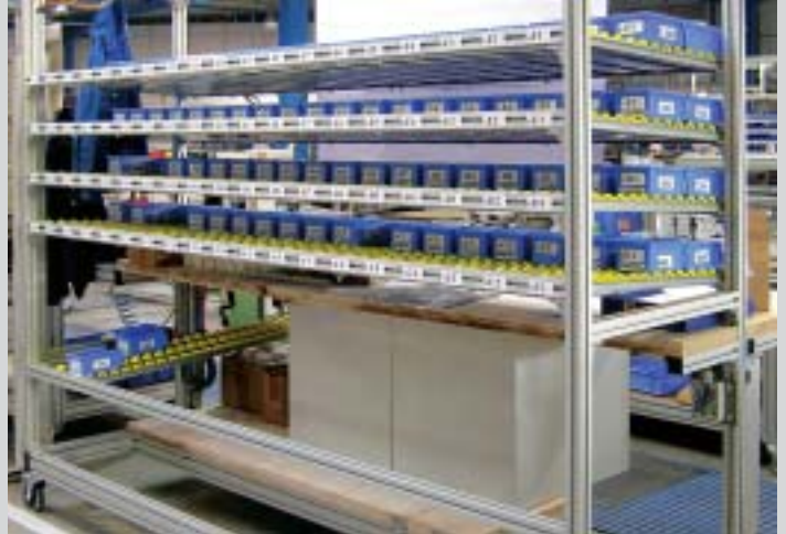
Kanban assembly workstation made of Series 40 profiles, flow rack for max 76 different products, workbench with hydraulic height adjustment
