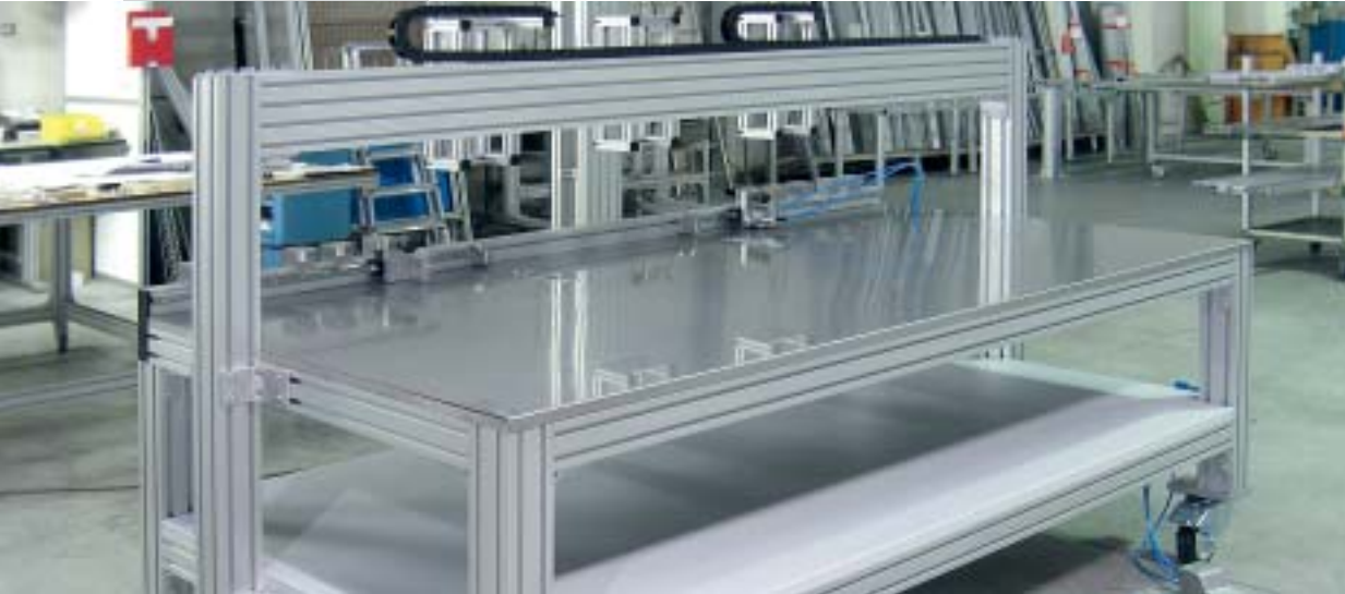
Customer-specific assembly table with linear track and pneumatic clamping
