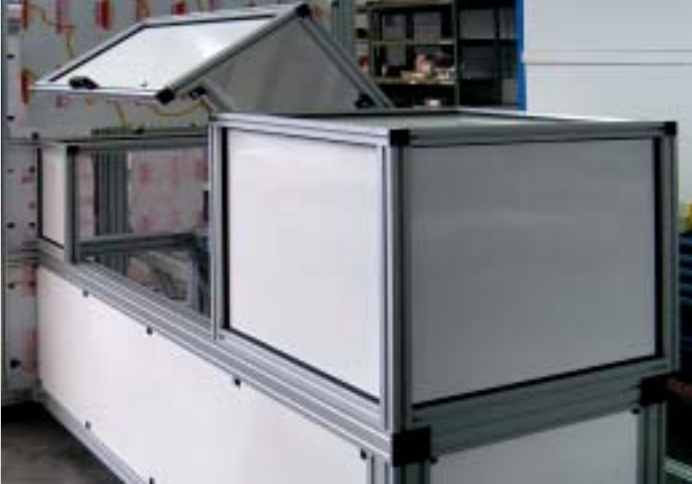
Machine guarding with vertically swinging door actuated by gas springs
