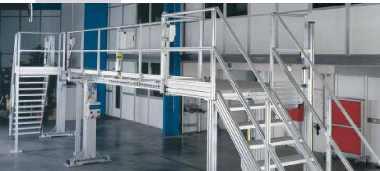
Assembly platform for helicopters. Air cushion floor elements enable effortless movement of the whole structure on the factory floor
