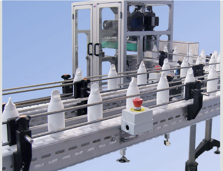
Linking via INOX flat top chain conveyor
