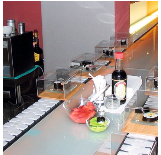
INOX flat top chain conveyor used in hospitality field
