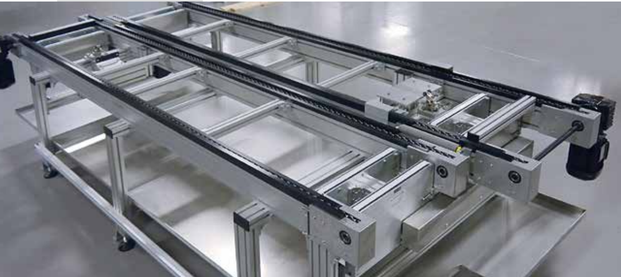
Versamove ultra: Customer-specific parallel circulation system with pallet transfers
